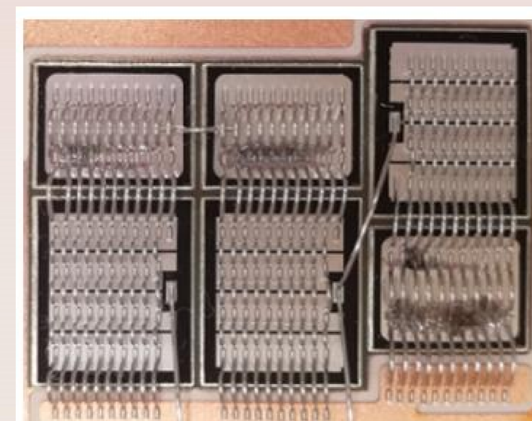
Surge current failure mode of the selected module
